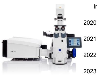
Laser-scanning confocal microscopes are commonly found as flagship instruments for shared access in light microscopy facilities.
